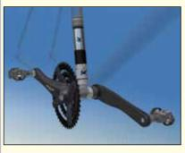
WORGL, Austria—Gruber's electric-assist, 200-watt motor is designed to fit within a 31.6-millimeter seat tube and drive a custom Hollowtech II-style bottom bracket axle through bevel gears. As long as the seat tube is straight and meets the bottom bracket shell close to the middle, the system will work. Since the system drives the crankset, it integrates seamlessly with a bike's drivetrain. The motor assist is turned on and off with a switch on the end of the handlebars. The en-
