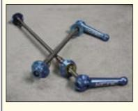
TUCSON, AZ—Lightweight quick-release skewers promise to shed grams in a relatively simple way, but they can be fiddly and slow down wheel removal. To remove weight many manufacturers cut down quick-release cam and washers so much that they can fall out of alignment when the lever is open. To keep its quick release light and easy to use, KCNC developed a ball-and-socket design that always remains in alignment when the skewer
