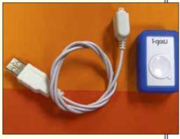
on Google Maps and Google Earth." It comes with a USB cable that connects to a PC for charging of the internal battery and for data transfer. The iGotU GPS Travel Logger retails for \$79.95. For more information, e-mail Cochrane at bill@coastal-cruisers.com.
