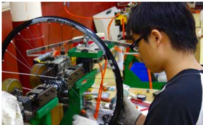
Workers at truing stands build up to 50 wheels a day each. All of American Classic's wheels are hand finished.
